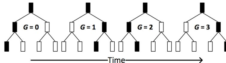
Figure 3: Reverse-lexicographic order of paths used by Algorithm 2. After path  $G = 3$  is evicted to, the order repeats.
